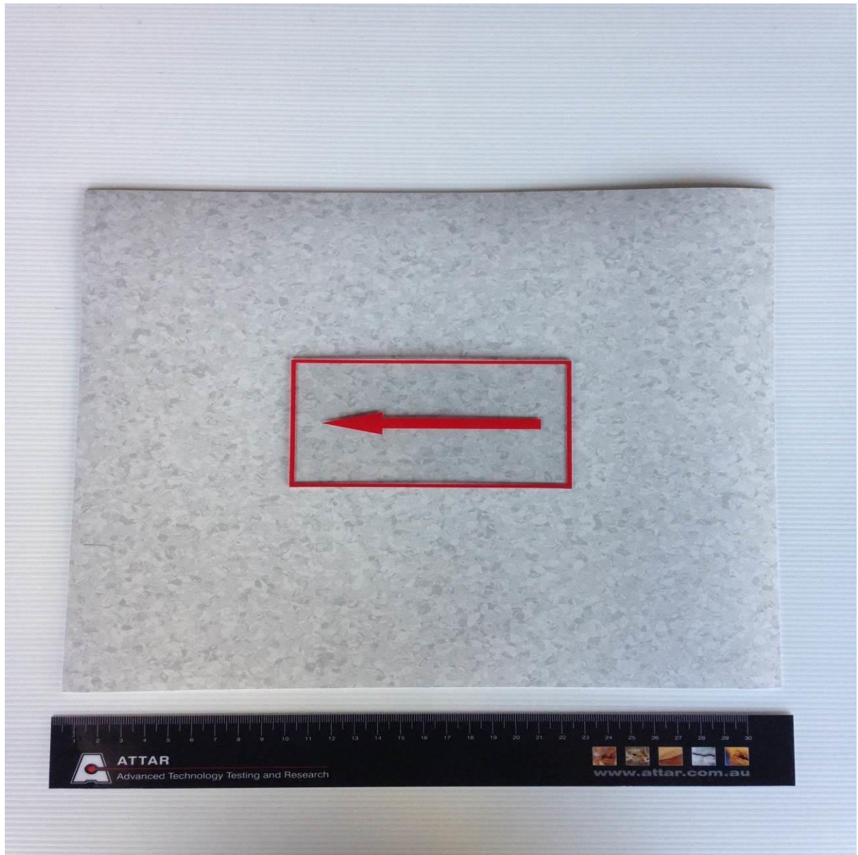
Figure 1: Primo SD – Highlighted area indicates area tested and direction of test.
